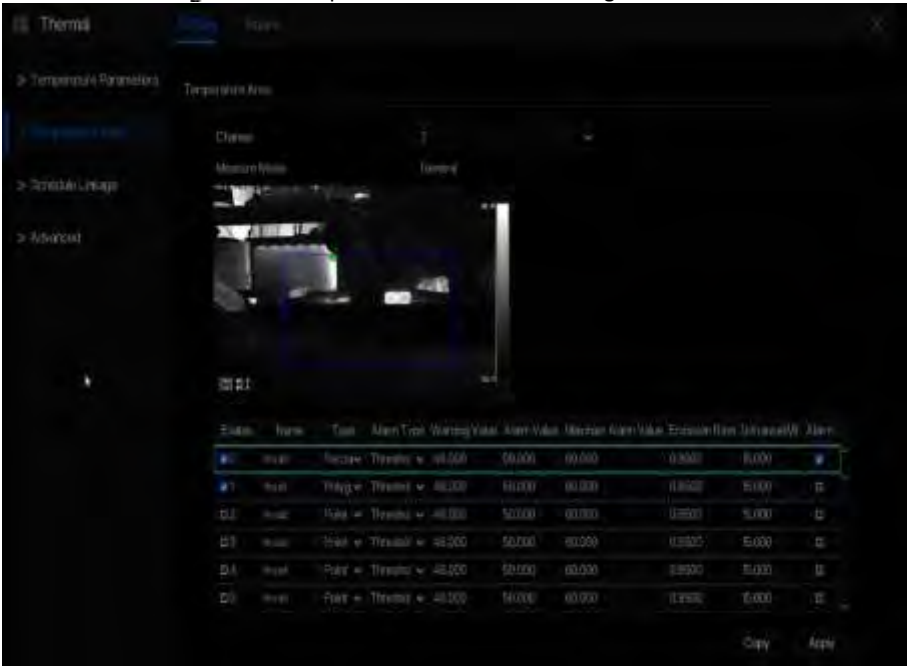
Figure 6-19 Temperature area and alarm configuration
